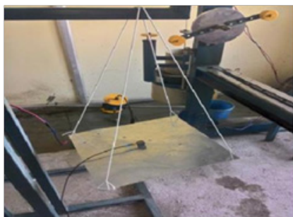
Figure 3. Modal test using FFT Analyzer
