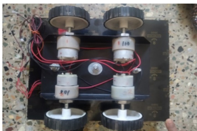
Figure 7: BLDC motors attached to wheels of car
